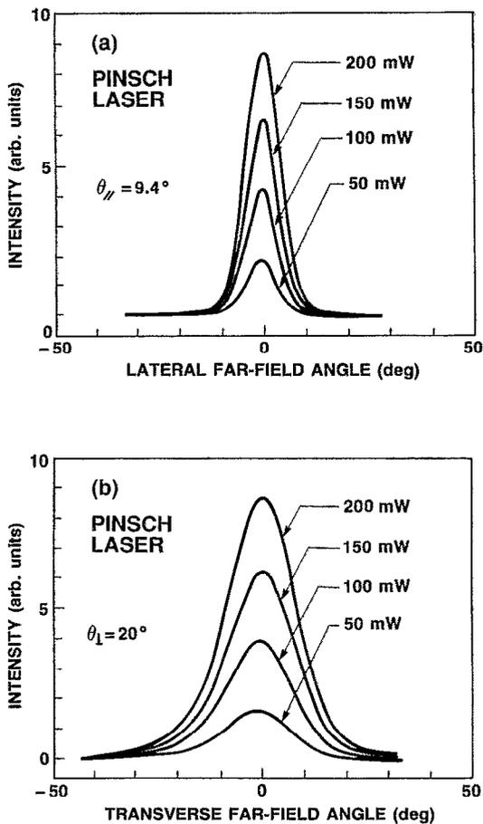
FIG. 3. The (a) lateral and the (b) transverse far-field patterns of the PINSCH laser at 50, 100, 150, and 200 mW. The FWHM angles are  $\theta_{\parallel} = 9.4^{\circ}$  and  $\theta_{\perp} = 20^{\circ}$ , respectively.
