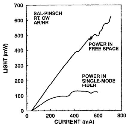
FIG. 4. The room-temperature CW  $L$ - $I$  curves of a  $5 \mu\text{m} \times 750 \mu\text{m}$  PINSCH laser for output power in free space and output power coupled into a single mode fiber with  $5 \mu\text{m}$  core diameter. The maximum powers in free space and in the fiber are 620 and 130 mW, respectively.
