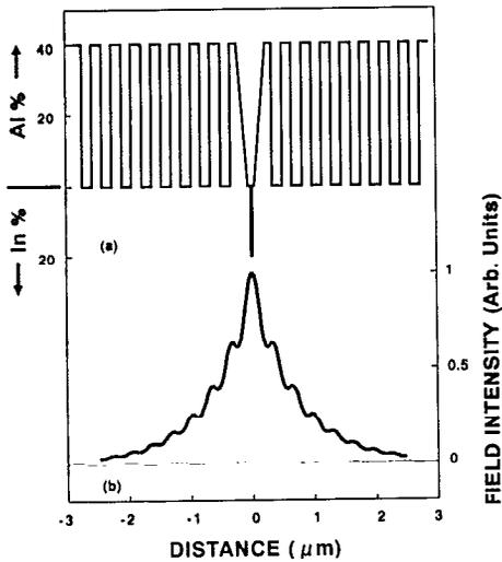
FIG. 1. (a) The layer composition of the PINSCH quantum well laser. (b) The calculated optical field distribution of the PINSCH laser.
